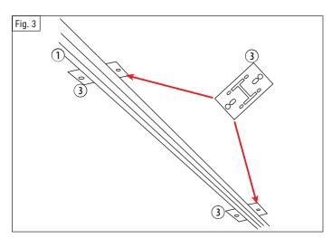
**Step 1:** The ceiling brackets (3) are already fixed to the floor with a distance of min. 45 cm to the rail end of the single slide rails (1).
