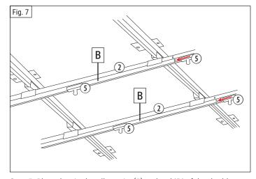
Step 5: Place the single roller units (5) on level 'B' of the double runners.After attaching the carriage rollers, attach one rail stopper (6) to each end of the slide rail with the fastening screw.
