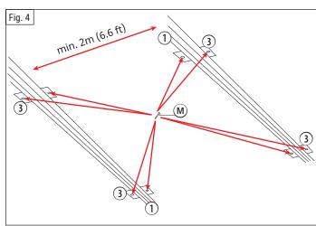
**Step 2:** Mount the two single slide rails (1) at a distance of about 2 m parallel to each other on the ceiling. To do this, screw the brackets (3) into the ceiling using two mounting screws\* of M6 size each (M) and suitable dowels/ceiling anchors\* if necessary.
