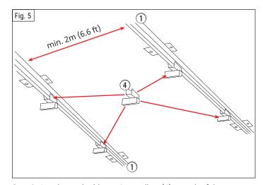
Step 3: Attach two double carriage rollers (4) to each of the two assembled single slide rails (2).
