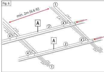
**Step 4:** Insert level 'A' rail of the double slide rails (2) into the lower part of each of the two double carriage rollers (4) so that they run crosswise under each of the two single slide rails (1). This results in a cross-like basic rail structure (see Fig. 6)
