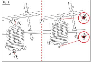
**Step 6:** Attach the pantographs (6) with their upper sockets (X) to the spigots (Y) of the single carriage rollers (5). Insert the spigot adapters (7) into the lower sockets (Z) of the pantographs. Handtighten the knob screws (10) on both sockets.
